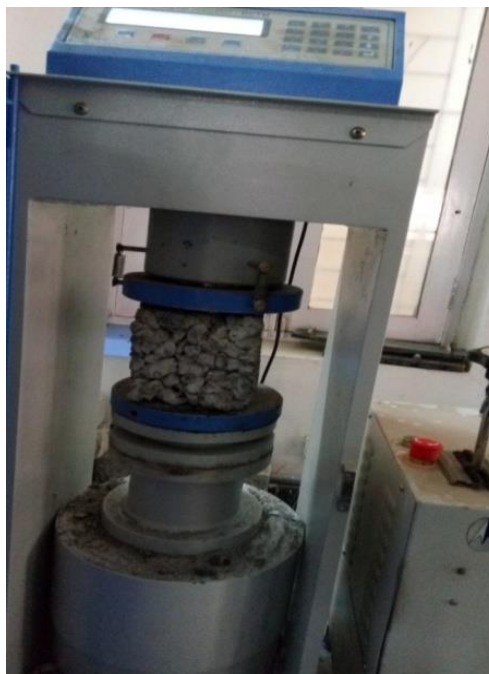
Fig. 1: Compressive strength test
